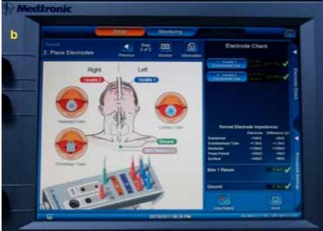
**Picture-5:** After the patient is intubated and the stimulating and recording connections are connected to the device via the connection box, on the screen a) control of connections of recording and stimulating electrodes, b) control of electrode resistances
