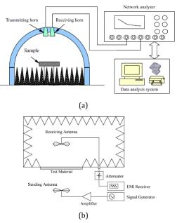
Figure 2. Spectrum analyzer and field generator measurement.
