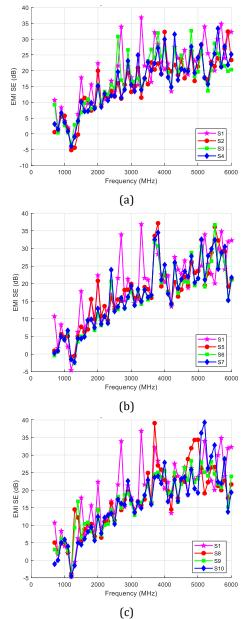
Figure 7. EMI SE values for composites (a)  $Fe_2O_3(325)$ , (b)  $Fe_2O_3$  (50 nm), and (c) FeO(OH) in the R position.
