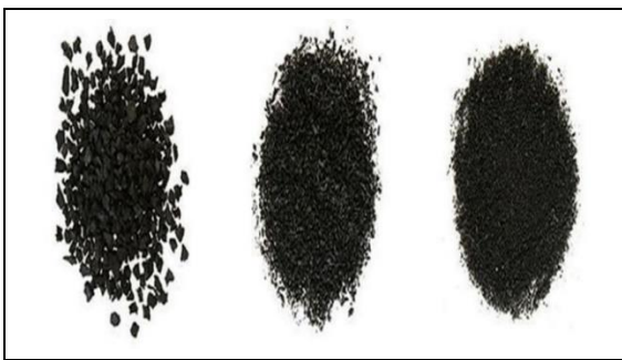
Figure 2. Types of waste tire rubber used in concrete [45].
