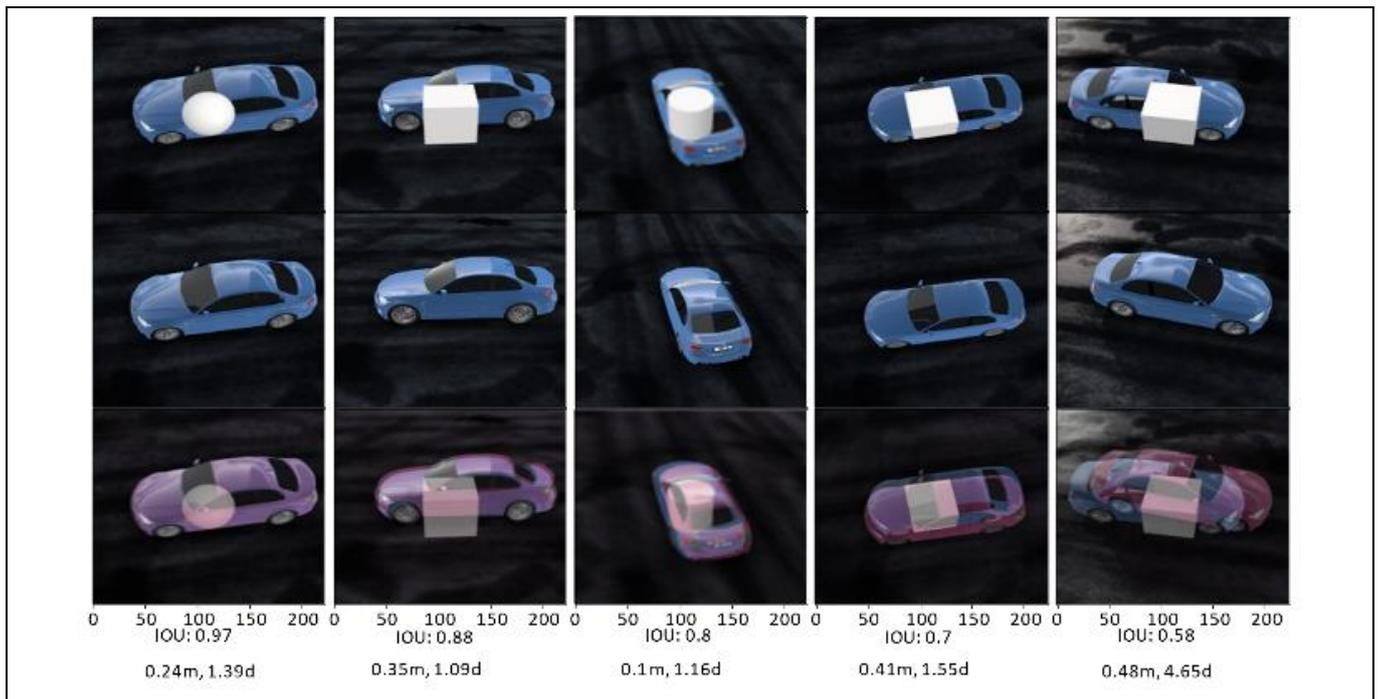
Figure 3. Archetypal representations for each IOU threshold. Top row represents the ground truth. Middle row is the view of the estimated camera location and orientation. Bottom row is the composite image of estimation and ground truth. Axis labels shows the IOU and the translation and the rotation error.
