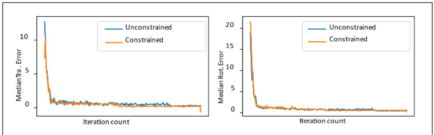
Figure 5. Median validation errors of PoseNet. Constrained quaternion curve shows the effect of exponential regularizer. Both translation and rotation error approaches local minima at faster rate, typically about 50%.
