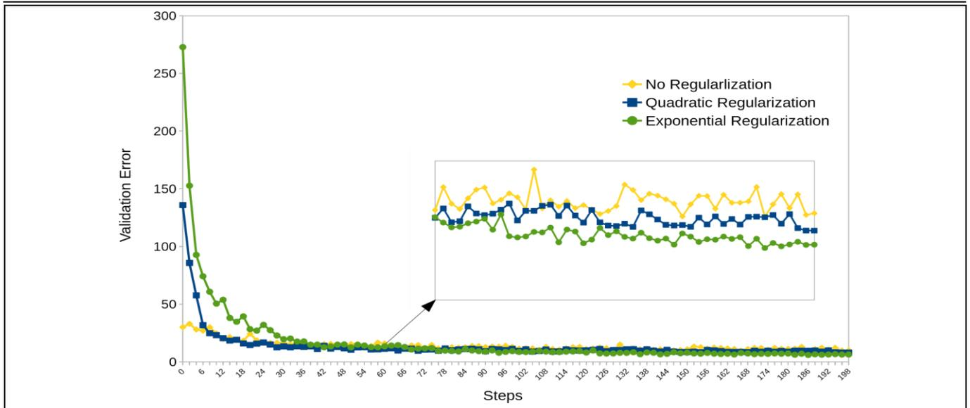
Figure 4. Effect of quaternion norm regularization on the validation loss. In the beginning of the training cumulative loss is significantly higher compared to the vanilla loss due to the chaotic estimations of the network. However, as the networks becomes more stable, constraint helps, optimization to find a slightly better minimum and faster convergence.
