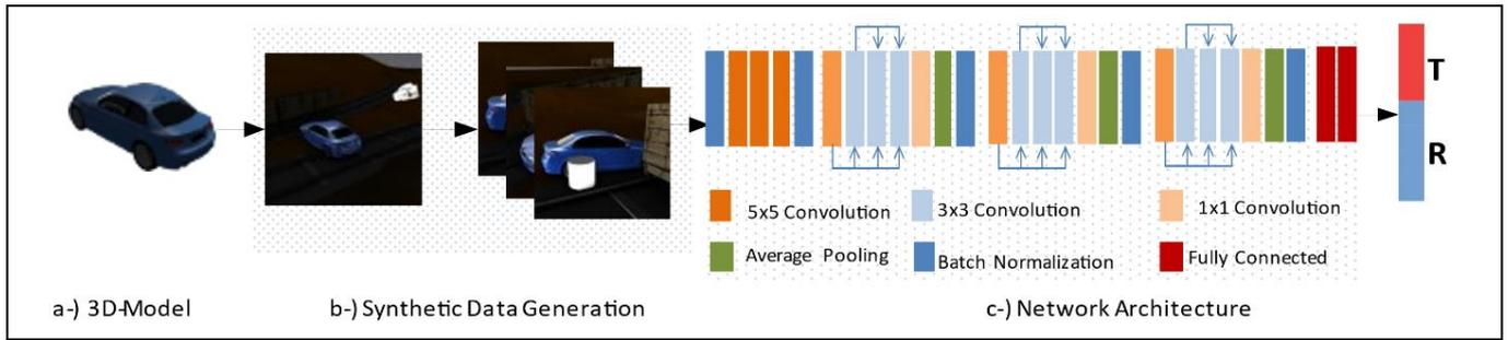
Figure 1. Direct estimation of camera poses with neural models using synthesized images. (a): Given a 3D model we generate random texture maps and distinct shapes and material properties. (b): We render images on dynamic and transparent backgrounds with varying illumination. Random 3D shapes and objects are placed between camera and the target object. (c): We train a custom densely connected custom neural architecture to directly estimate either camera or target object pose.
