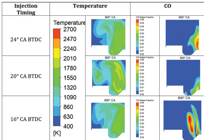
Figure 9. Combustion Chamber Temperature and CO Emissions
