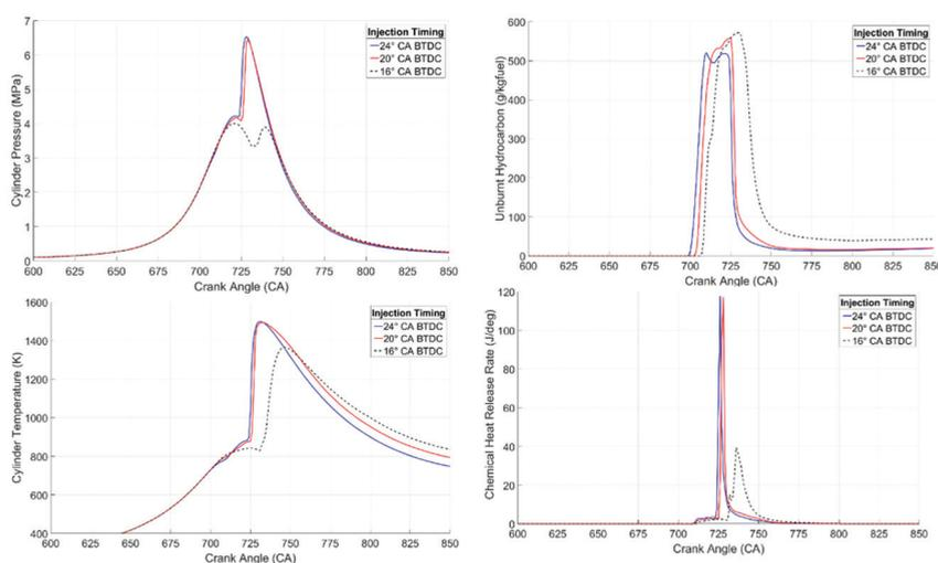
**Figure 5.** Motor Performance Parameter for 20° CA Injection Duration
