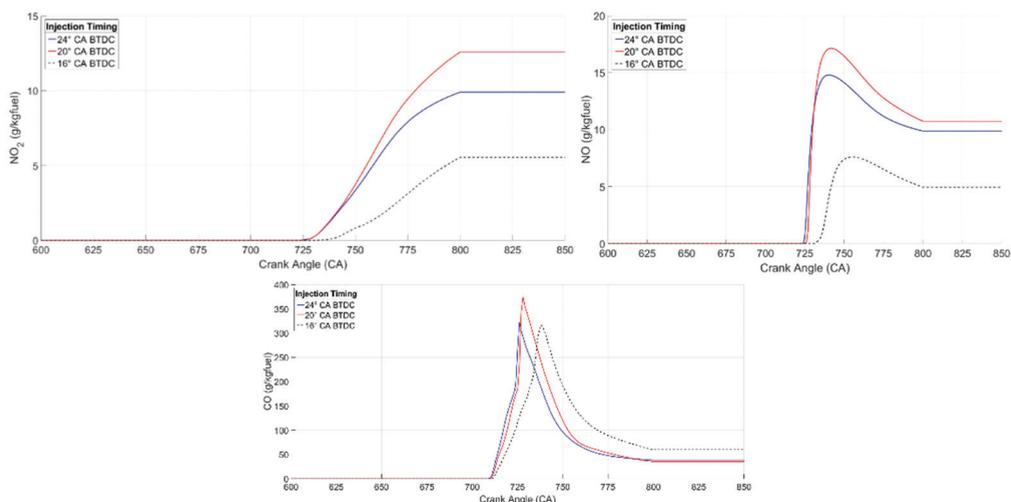
Figure 7. NO<sub>x</sub> and CO Emissions for 20 CA Injection Duration
