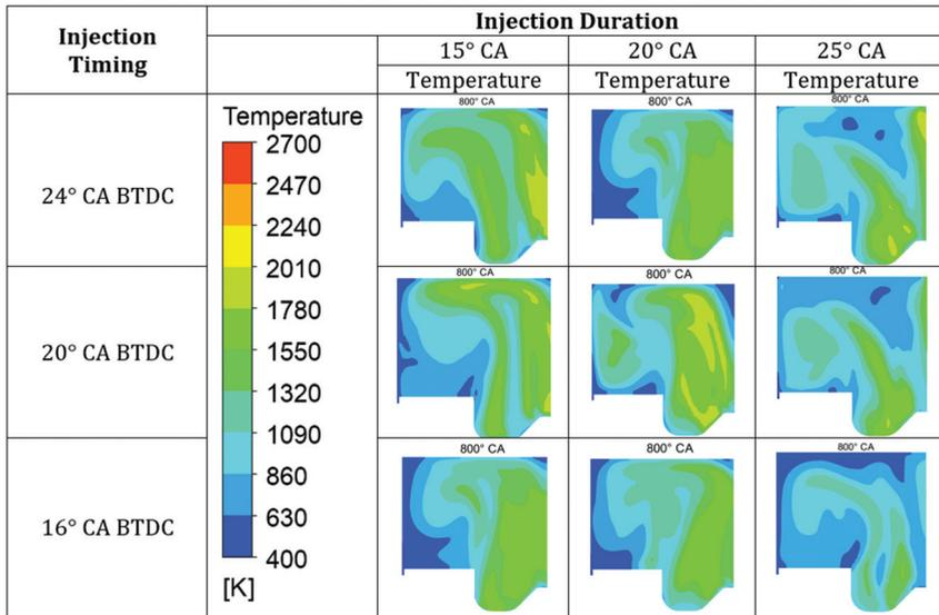
Figure 10. Combustion Chamber Temperature for Different Injection Duration
