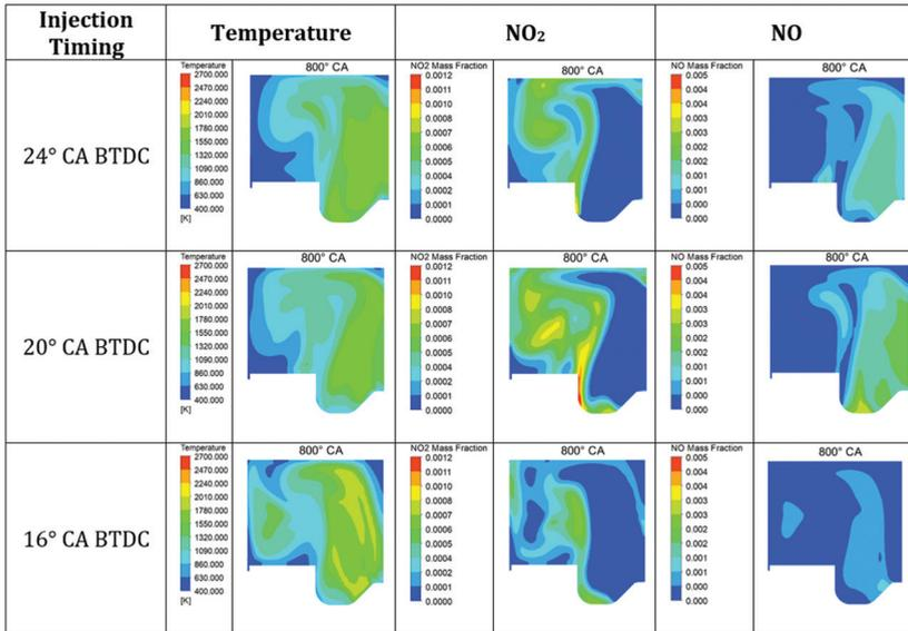
Figure 8. Combustion Chamber Temperature,  $NO_2$  and NO Emissions
