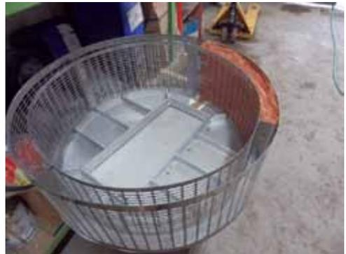
**Figure.7** Turbocharger outer filter prototype product.
