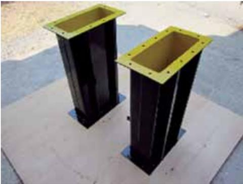
**Figure.8** Manufactured distance units.
