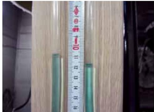
**Figure.11** Visual pressure drop measurement, U-manometer.
