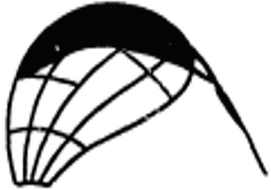
**Figure 7.** Comparison of Cavity Pattern with Experiments,  $J=0.7$ ,  $\sigma=1.715$  (DTMB 4382) (Left: Present Method, Right: Experiment taken from [21])
