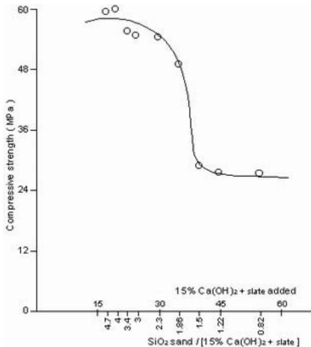
Figure 3: Variation of compressive strengths at 4-5 hours of Ca(OH)<sub>2</sub> and rice husk ash-activated hydrothermal products versus SiO<sub>2</sub> sand / (15% Ca(OH)<sub>2</sub> + RHA) ratio.
