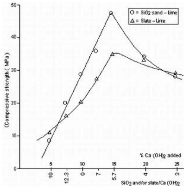
A maximum strength of 47.6 MPa is obtained after 4.5 hours autoclaving and 15%  $\text{Ca}(\text{OH})_2$  content (silica sand/ $\text{Ca}(\text{OH})_2$ =5.67) while in our earlier investigation (1) the maximum strength of 25.8 MPa was recorded after 48 hours autoclaving at a steam pressure of 0.1 MPa (100°C) and 30.0% lime content.
