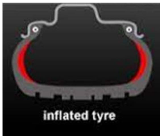
Figure 2 Tubeless tyre (inner profile of car rim)
