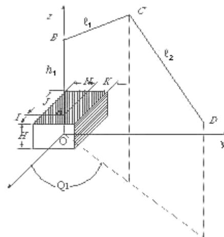
In what follows, a three-link arm is considered, as shown in Figure 1, with three revolute joints. Work space constraints are set and relationships are formulated that enable the determination of link dimensions to meet the constraints. Likewise, relationships are set up between locations of the work piece and displacement variables.
