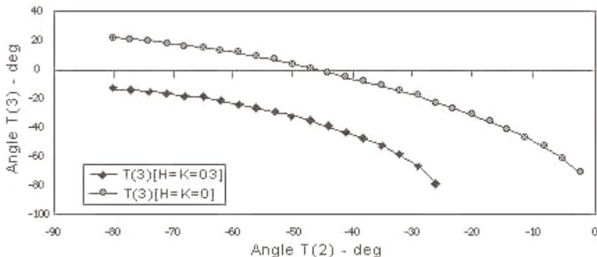
respectively, with  $\theta_2$  for operations at platform level. It is noted once again in Figure 8 that there are two possible reaches for number of T(2) angles. The reach at ground level varies from 0.3 m to 0.6 m and 0.05 to 0.25 m for the two possible modes of operation. The reach at platform level is considerably more covering the range from 0 to about 1.1 m between the two modes of member CD. The ranges of operation of both angles are again observed to be about 90°.
