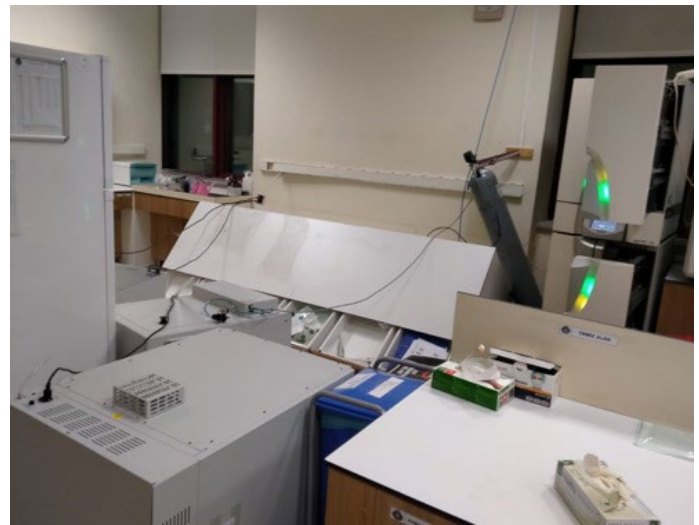
Figure 3. Damage to equipments in the microbiology laboratory at the Department of Microbiology, Kahramanmaraş Sütçü İmam University Hospital following the earthquake (photo by Dr. Filiz Orak).
