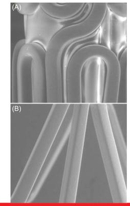
Figure 2. SEM images of (A) crimped and (B) expanded Tetrilimus stent.
