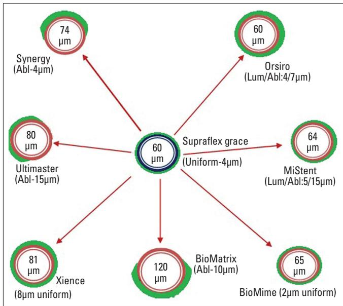
**Figure 1.** Schematic representation of strut and polymer thickness of contemporary stents. Green color indicates the thickness of the polymer
